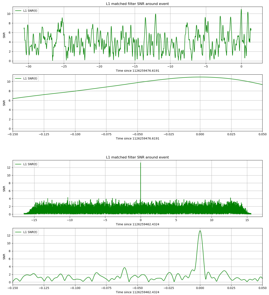
Figure 6. Non-optimal (top) and optimal (bottom) matched filtering for L1 for the event
